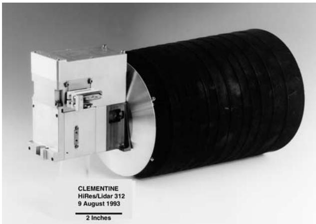
**Figure 1.** Photograph of Clementine HIRES camera (courtesy Lawrence Livermore National Laboratory).
